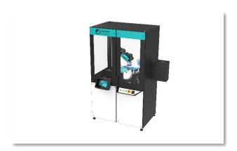
Caption: Solution Kit Part Separation with 2D Grasping-Kit: new automation solution for vision-based part separation with the Al-supported industrial robot HORST600, the SCHUNK 2D Grasping-Kit and the FlexiBowl parts separator.
