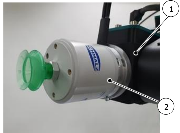
Fig. 6-17: Fastening the basic unit in the base
