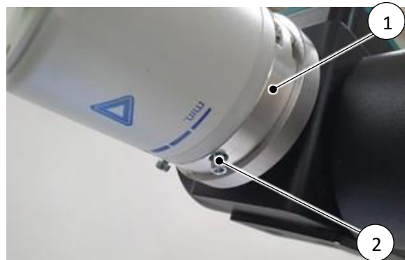
Fig. 6-18: Fixing the vacuum gripper
