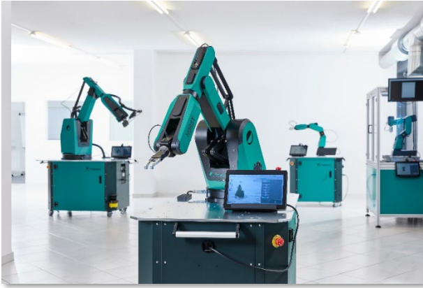
Caption: fruitcore robotics' product portfolio includes three models of the Digital Robot HORST with 600 - 1,400 mm range and up to 12 kg load capacity.
