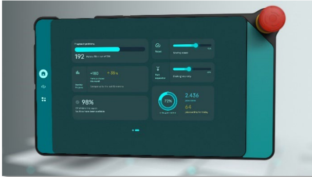
Caption: The entire application is controlled and monitored from a single point of control. With the customizable dashboard, the user always keeps an eye on the productivity of the annex and also has the option of making frequently adjusted parameters quickly and directly accessible.
